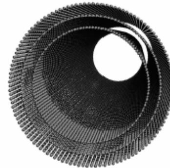
Figure 3.1b Schematic of a multi-walled carbon nanotube (MWNT)
